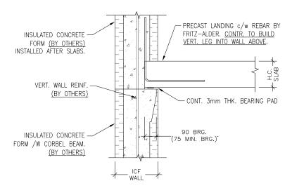
NOTE: ALL BEARING SUPPORT TO BE DESIGNED AND PROVIDED BY OTHERS PRIOR TO INSTALLATION OF HOLLOW CORE ON SITE
