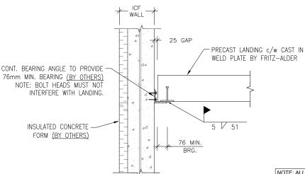
NOTE: ALL BEARING SUPPORT TO BE DESIGNED AND PROVIDED BY OTHERS PRIOR TO INSTALLATION OF HOLLOW CORE ON SITE
